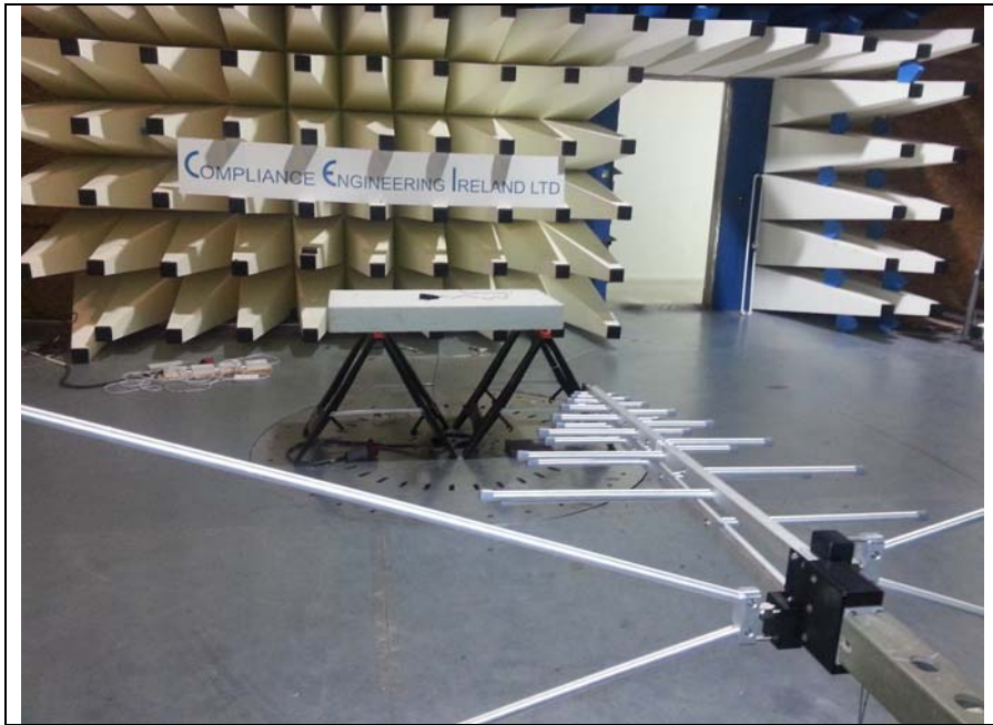
Fig 1 Test setup 30MHz -1GHz Rad Emission
