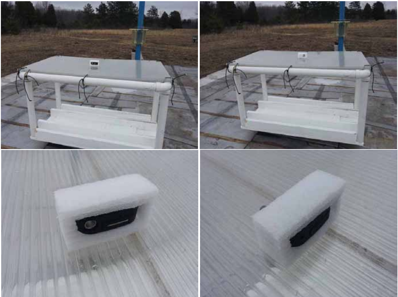
Figure 4: Radiated Emissions Test Setup Photograph(s).
