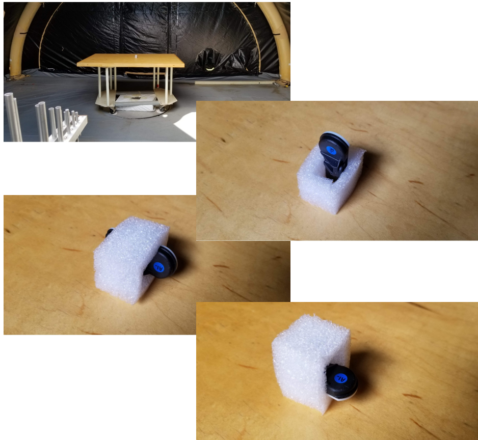
Figure 4: Radiated Emissions Test Setup Photograph(s).
