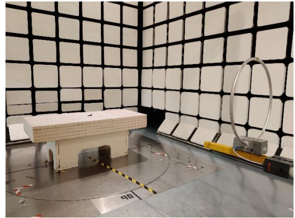
Radio-frequency radiated emissions (9 kHz -30 MHz).
