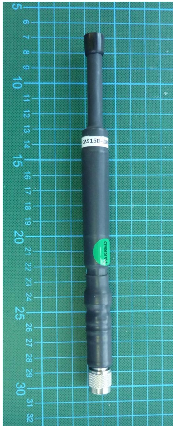
172629_24.jpg: CA915H antenna
