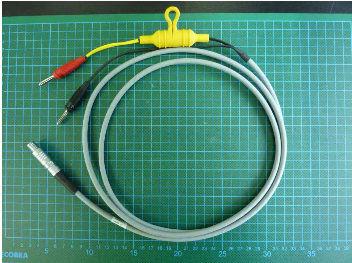
160575_28.jpg: DC power cable
