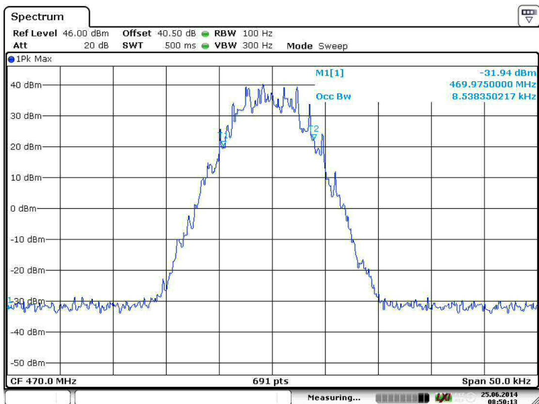
Figure 23. Mid channel 99% Occupied Power Bandwidth.
