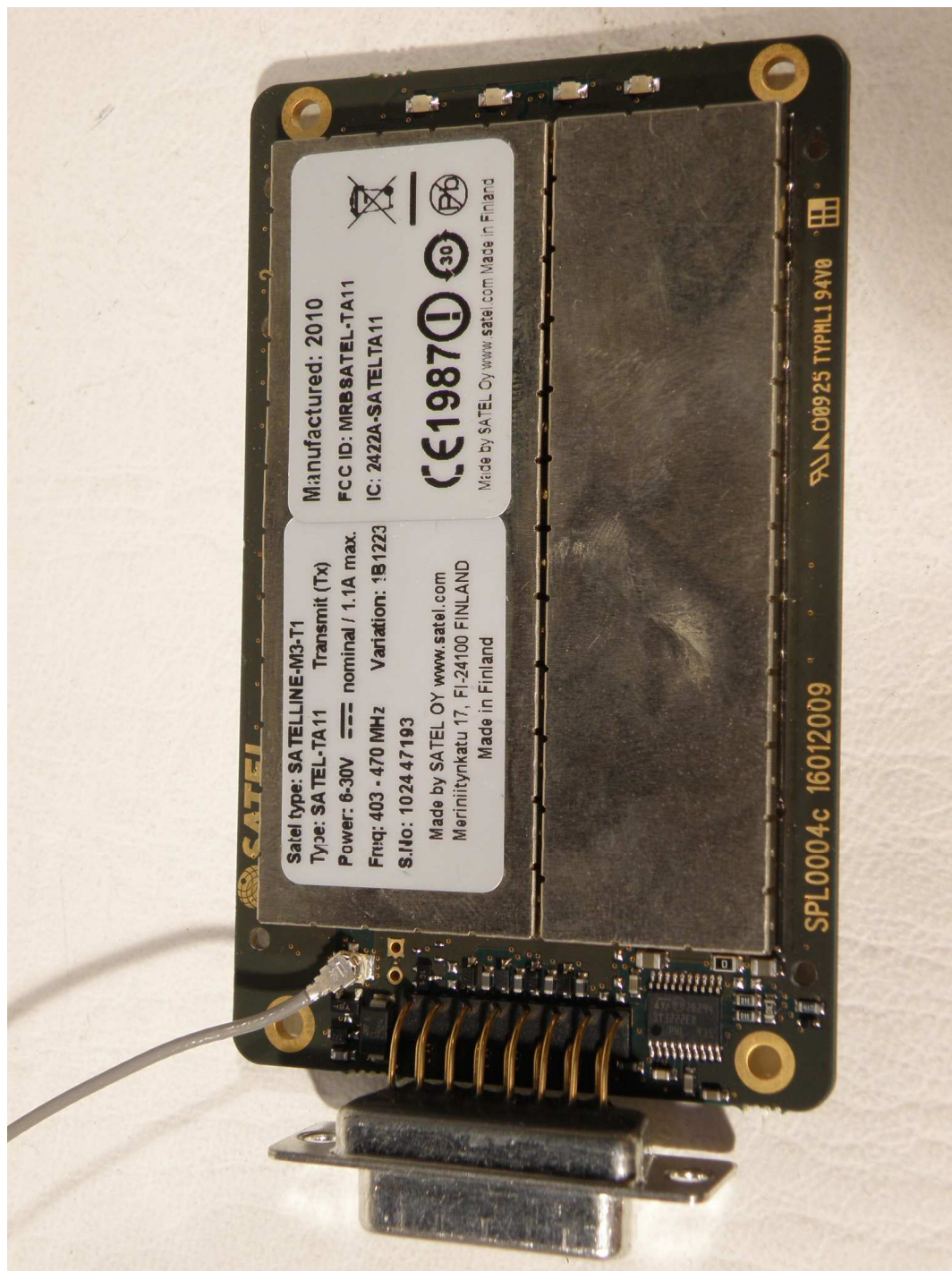
Photograph 1.: Upside with RF shield
