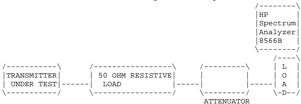
REQUIREMENTS: Emissions must be  $43 + 10\log(P_o)$  dB below the mean power output of the transmitter.
