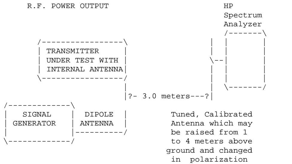
Equipment placed 1 meter above ground
