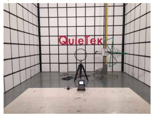
Description: Test Setup for 30MHz~1GHz
