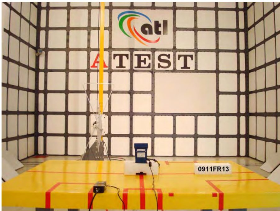
Description : Back View of Field Strength of Spurious Radiation Test Below 1GHz
