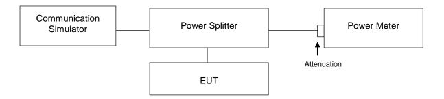
For the actual test configuration, please refer to the attached file (Test Setup Photo).
