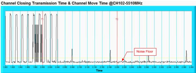
NOTE: An expanded plot for the device vacates the channel in the required 500ms.
