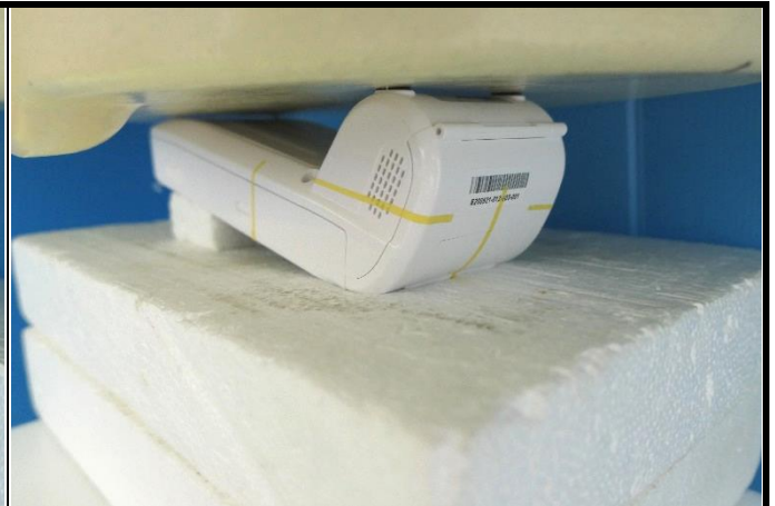
Rear Face of EUT at 0 mm
