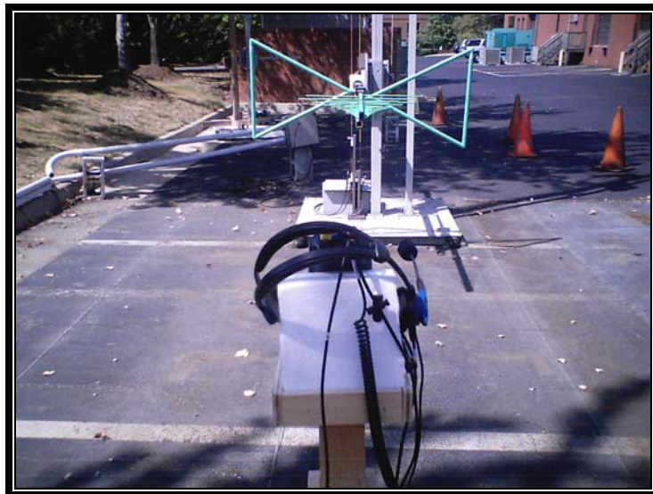
Photograph 4: Radiated Testing – Back View
