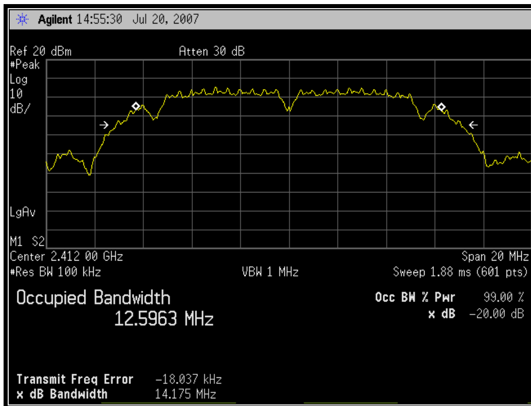
Plot 10-1: 99% Bandwidth Channel 1 (TX Frequency: 2412 MHz)
