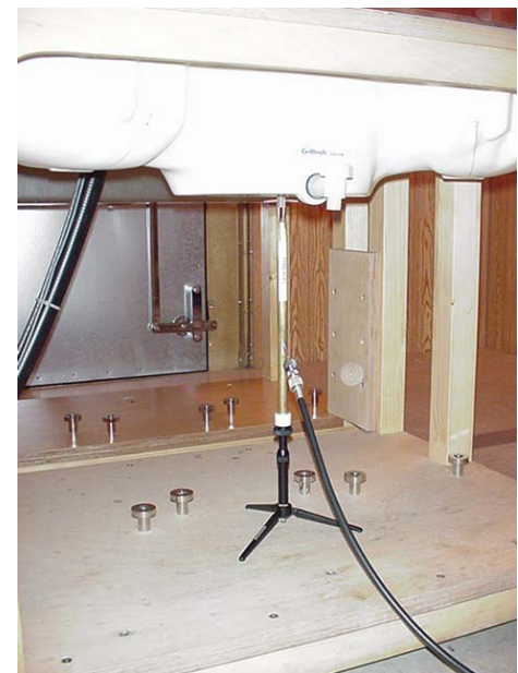
2450MHz Dipole Setup
