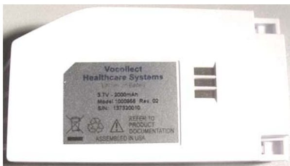
DUT Battery (Lithium-ion Model: 1000956 Rev. 02)
