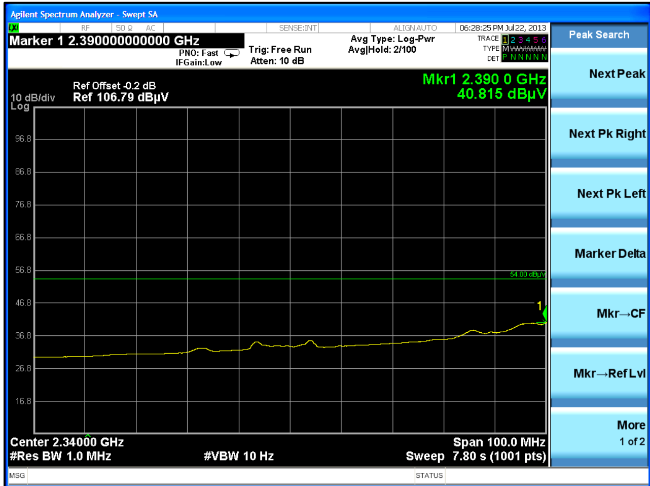
Plot 4-2: Lower Band Edge Average: 802.11b (11 Mbps)
