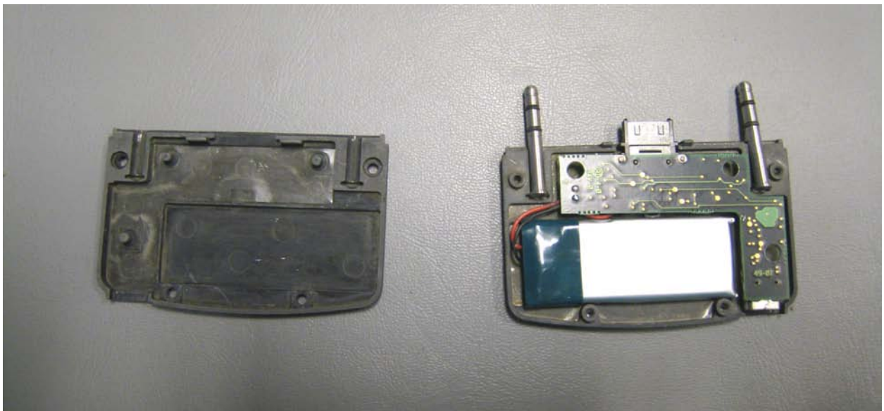
MOLE Battery Module, Internal, PCB bottom
