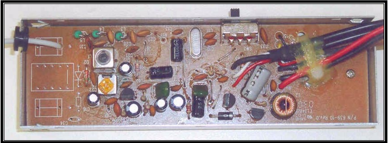
PHOTOGRAPH 8: COMPONENT SIDE OF FM-10 Tx MAIN PCB
