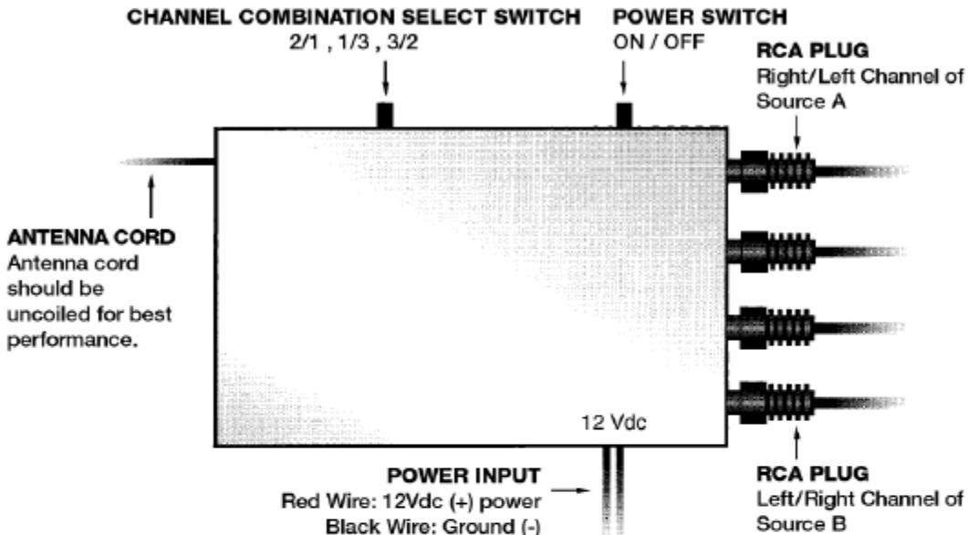
Audio input can be connected to either low-level fixed audio output or a variable level audio output (such as a speaker or headphone output). If it is connected to a low-level output, only the volume control on the earphones needs to be adjusted to control volume level. If connected to a variable level output, volume adjustment needs to be done at both the source and at the headphones.
