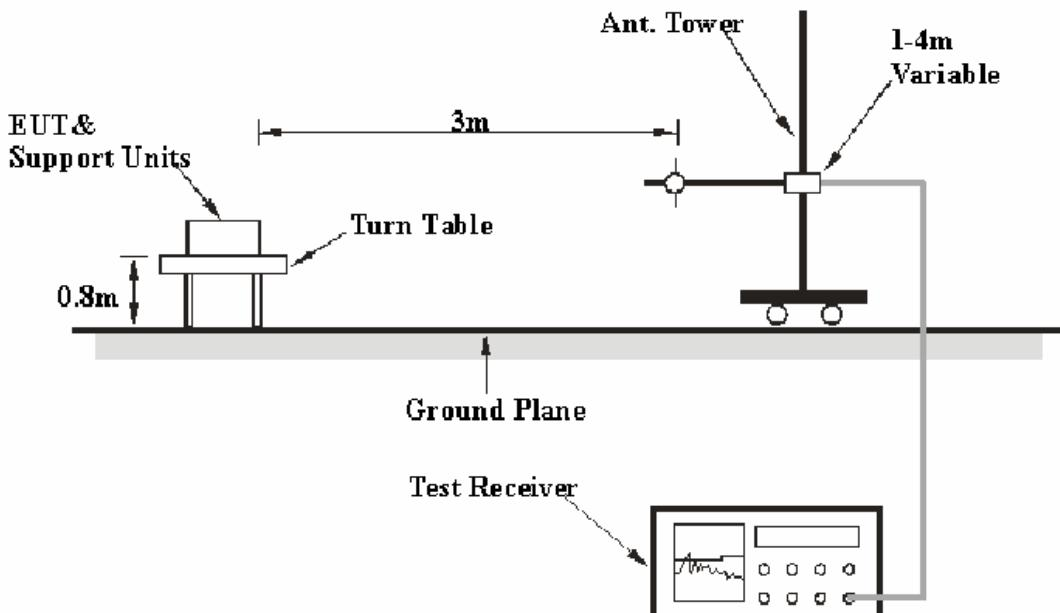
The radiated emission tests were performed in the 3 meters chamber B test site, using the setup accordance with the ANSI C63.4-2003. The specification used was the FCC 15.209, and FCC 15.247 limits.
