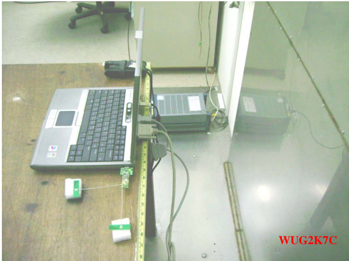
Photo 2: Conducted Emission Test Set-up photo
