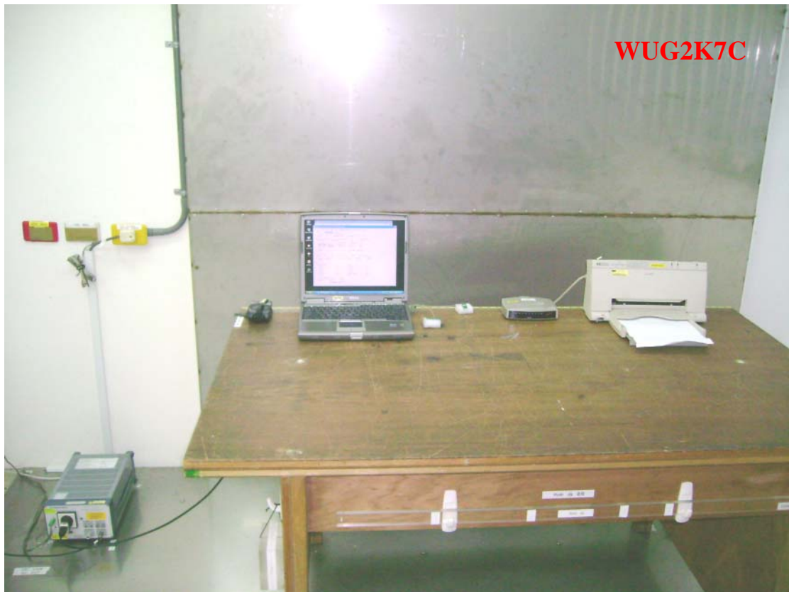
Photo 1: Conducted Emission Test Set-up photo
