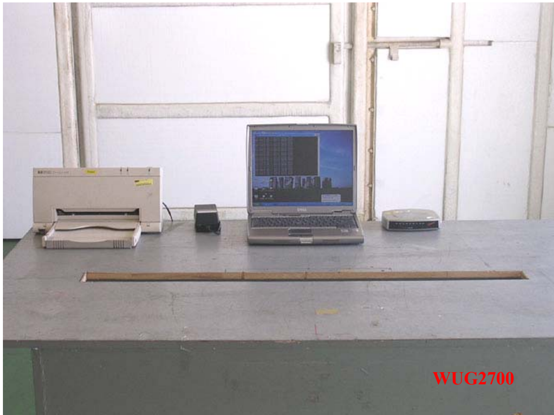
Photo 1: Radiated Emission Test set-up photo
