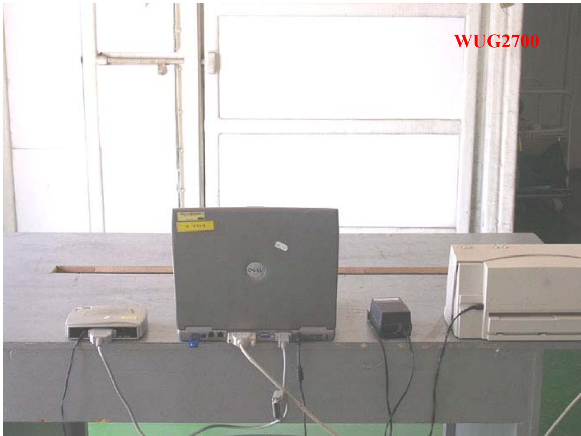
Photo 2: Radiated Emission Test set-up photo
