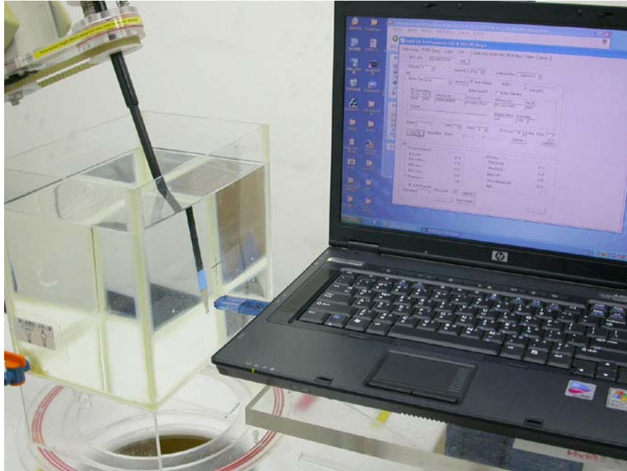
Figure 4: EUT perpendicular to phantom, 0 mm separation
