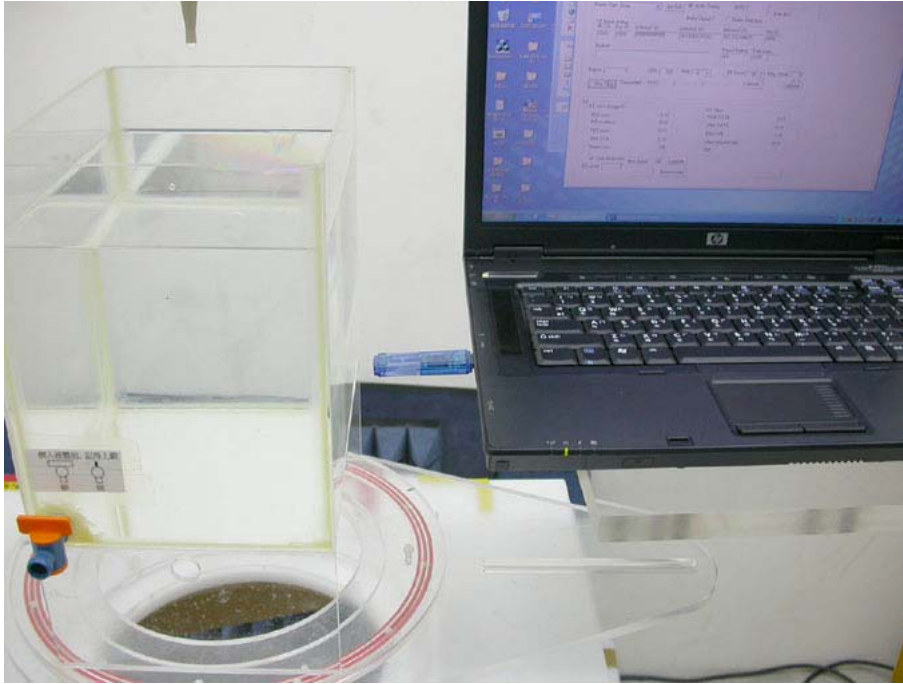
Figure 4: EUT perpendicular to phantom, 15 mm separation
