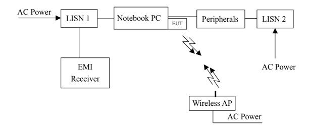
The EUT are connected to the main power through a line impedance stabilization network (LISN). This provides a 50 ohm/50uH coupling impedance for the measuring equipment. The peripheral devices are also connected to the main power through a LISN that provides a 500hm/50uH coupling impedance with 500hm termination.
