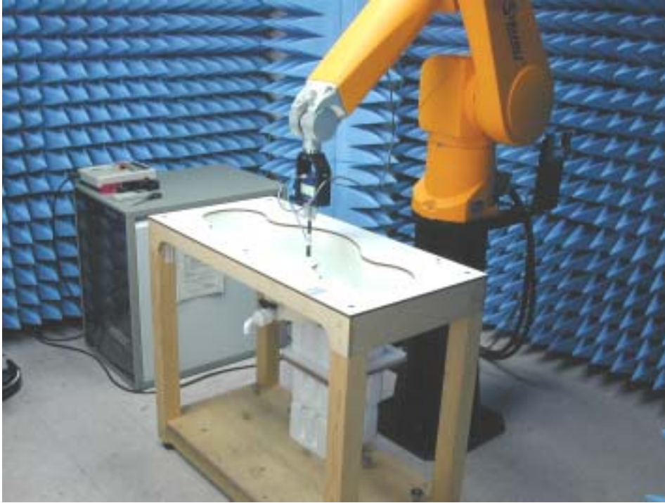
Fig.1 Photograph of the SAR measurement System
