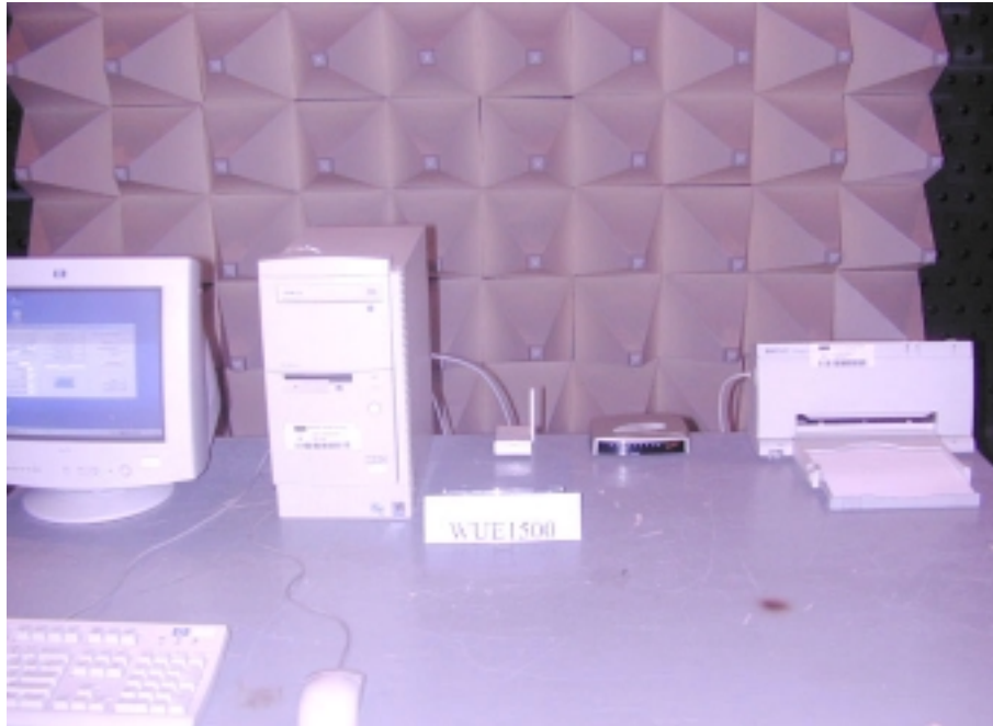
Photo 2: Spurious Test Set-up (rear)
