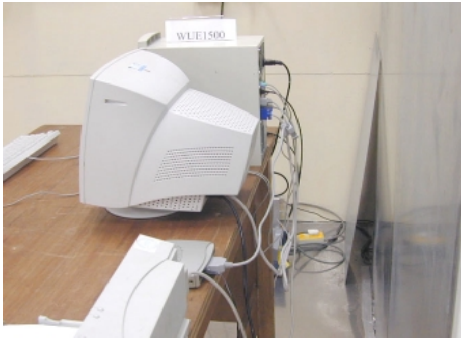
Photo 2: Conducted Test Set-up (rear)
