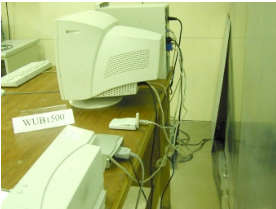
Photo 2: Conducted Test Set-up photo
