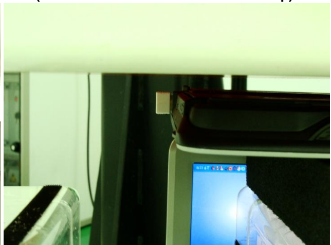
Direct Laptop Plug-in for USB Configuration 1 (for Back Off SAR) (Vertical Back with Phantom 10 mm Gap)
