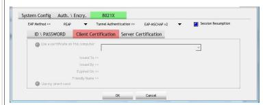
Users can select **Use a certificate on this computer**, a client certificate for server authentication. Or users can select **Use my smart card** to enable the Client Certification function.
