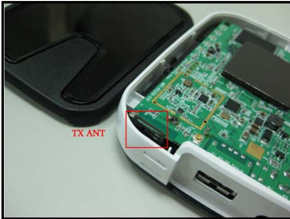
DESCRIPTION OF ANTENNA LOCATION
