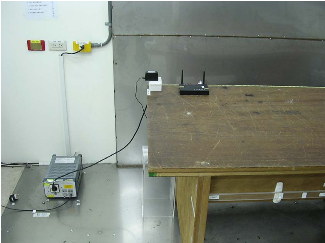
Photo 1: Conducted Emission Test Set-up photo
