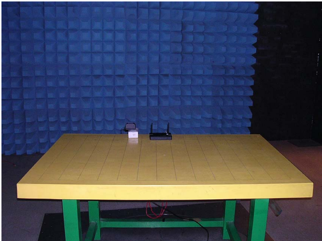
Photo 2: Radiated Emission Test set-up photo
