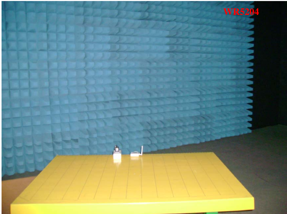
Photo 1: Radiated Emission Test set-up photo
