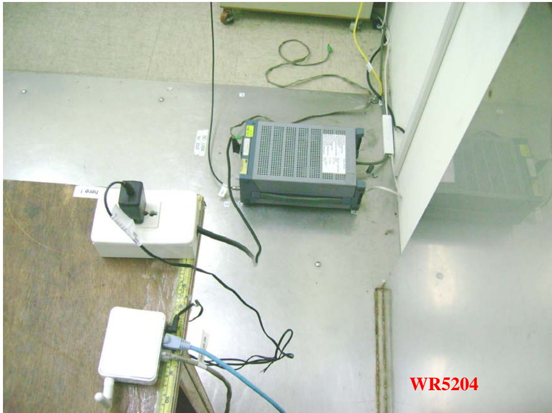
Photo 2: Conducted Emission Test Set-up photo
