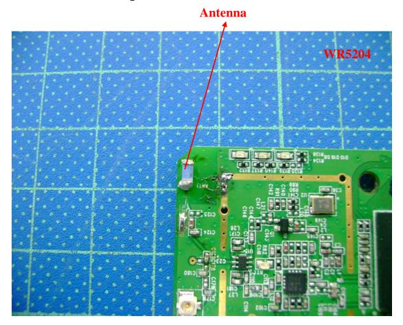
Photo 10: Internal photo of EUT with ceramic antenna
