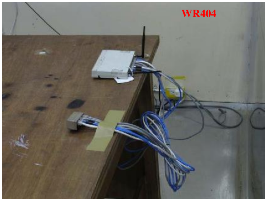
Photo 2: Conducted Emission Test Set-up
