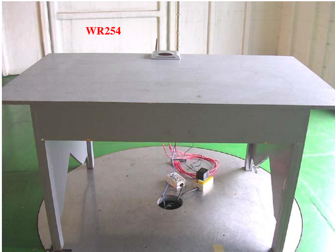
Photo 1: Radiated Emission Test Set-up
