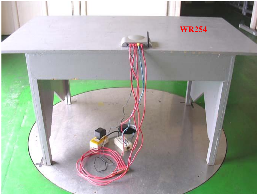
Photo 2: Radiated Emission Test Set-up
