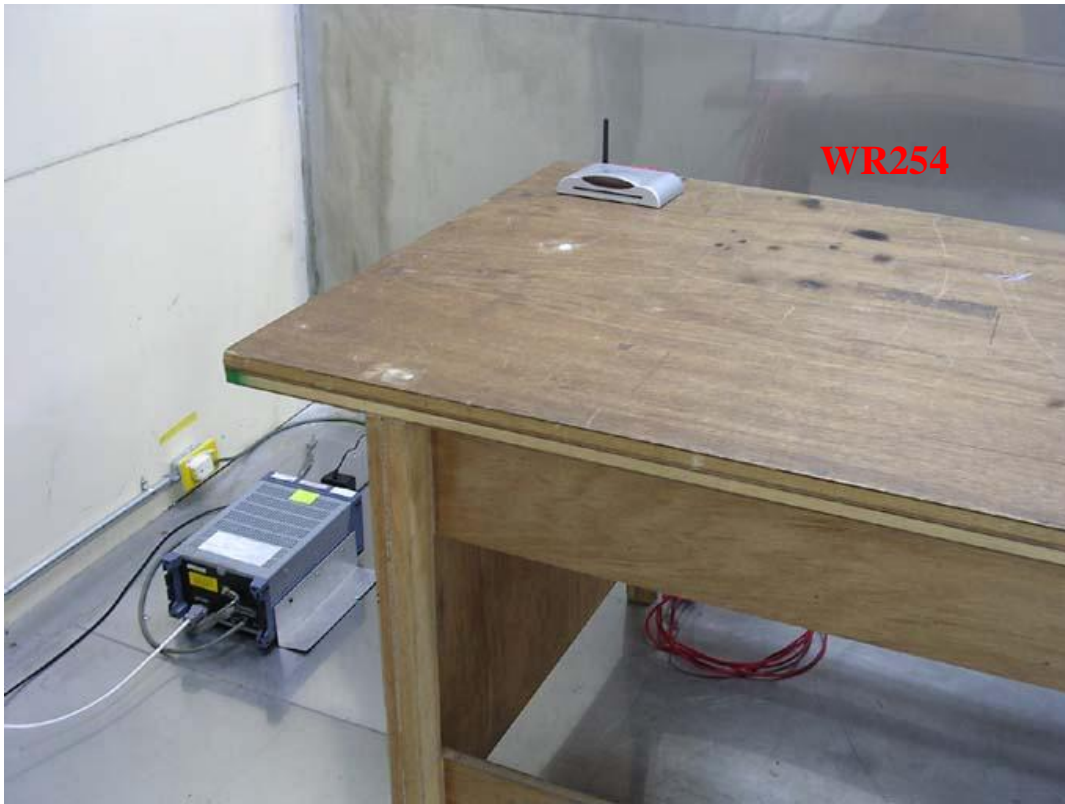
Photo 1: Conducted Emission Test Set-up
