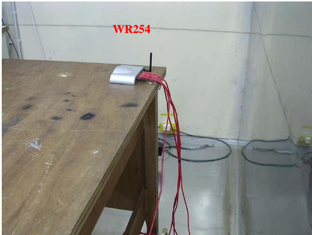
Photo 2: Conducted Emission Test Set-up
