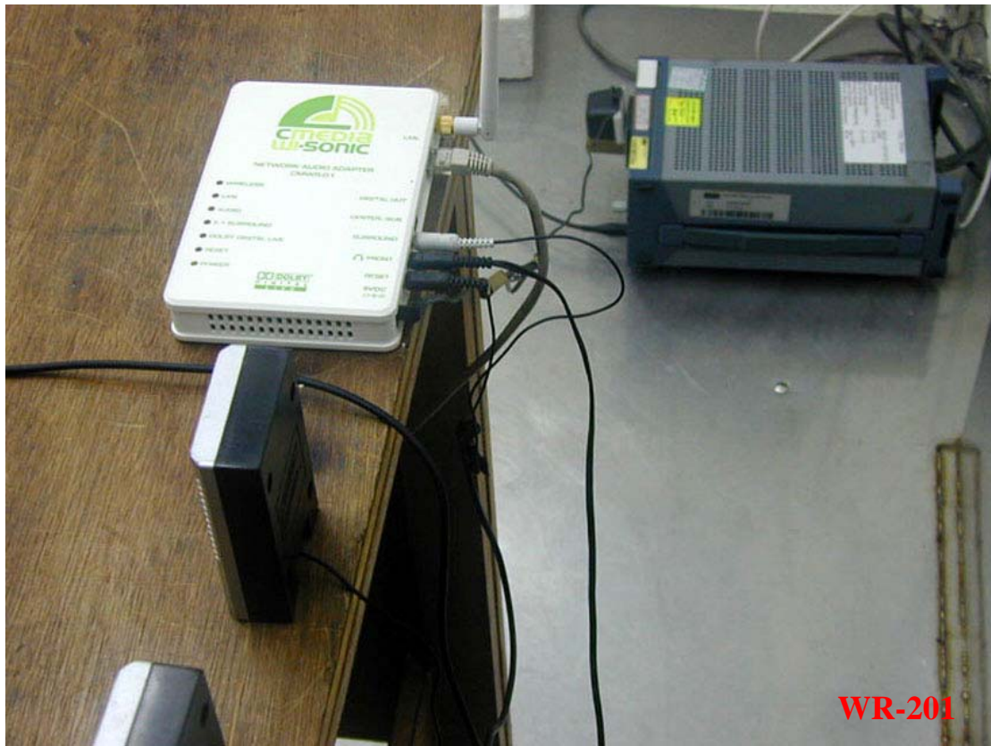
Photo 2: Conducted Emission Test Set-up photo
