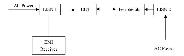
The EUT are connected to the main power through a line impedance stabilization network (LISN). This provides a 50 ohm/50uH coupling impedance for the measuring equipment. The peripheral devices are also connected to the main power through a LISN that provides a 50ohm/50uH coupling impedance with 50ohm termination.
