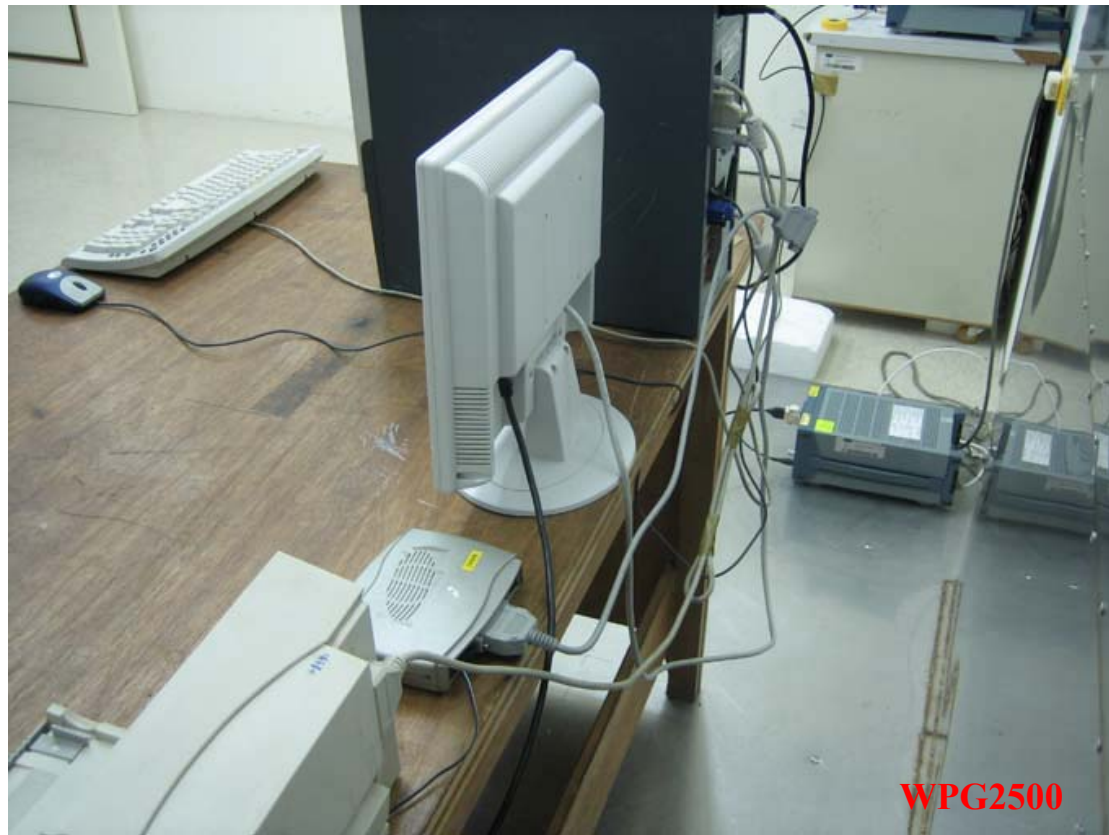
Photo 2: Conducted Emission Test Set-up
