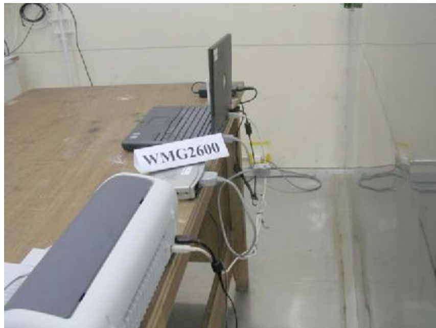
Photo 2: Conducted Emission Test Set-up
