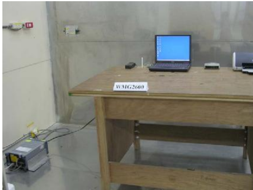
Photo 2: Conducted Emission Test Set-up
