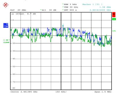
Power Density Plot on Configuration IEEE 802.11b Ant. A + Ant. B + Ant. C / 2462 MHz
