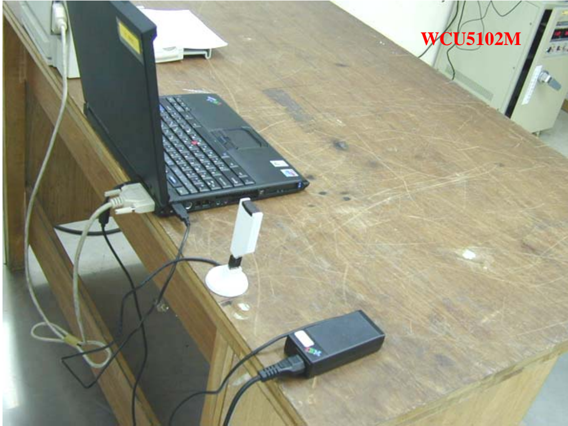
Photo 2: Conducted Emission Test Set-up
