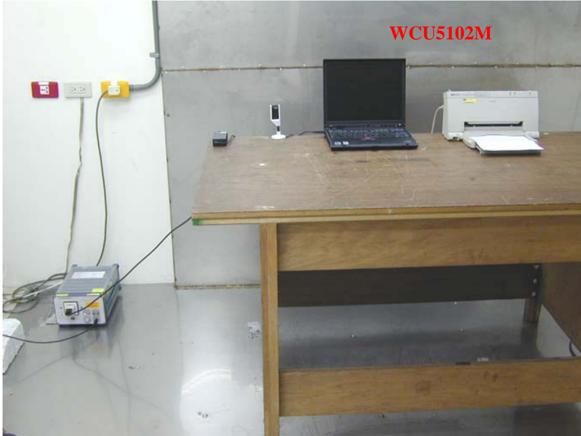
Photo 1: Conducted Emission Test Set-up
