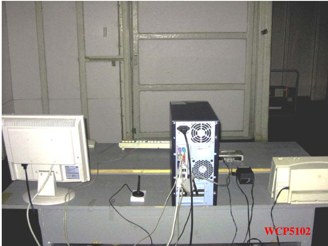
Photo 2: Radiated Emission Test Set-up
