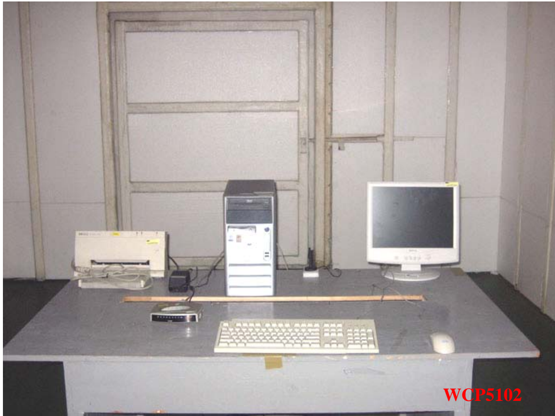
Photo 1: Radiated Emission Test Set-up
