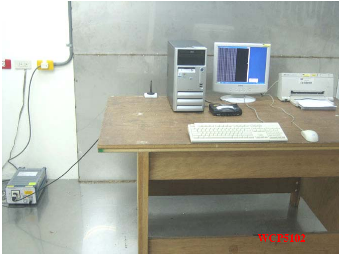
Photo 1: Conducted Emission Test Set-up
