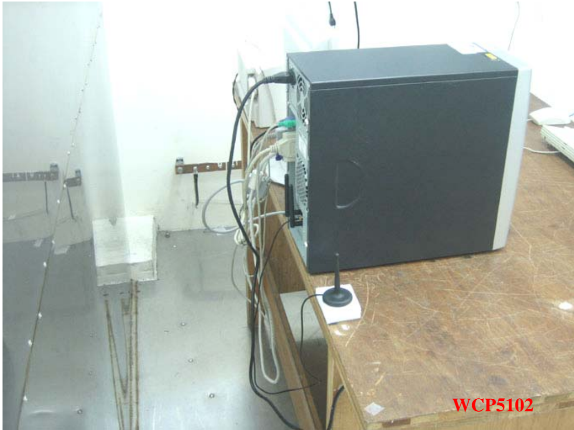
Photo 2: Conducted Emission Test Set-up
